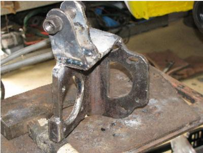
The final piece of the front end puzzle was squeezing a shock absorber mounting onto the top wishbone behind the top Rose joint. I had a single new Gabriel shock, from a mini, which we
